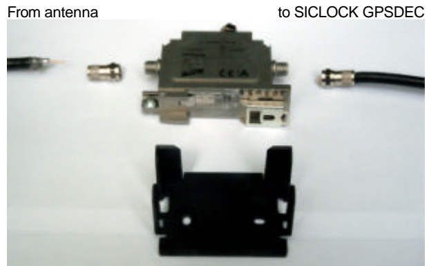
Fig. 3 Connecting antenna cable.
